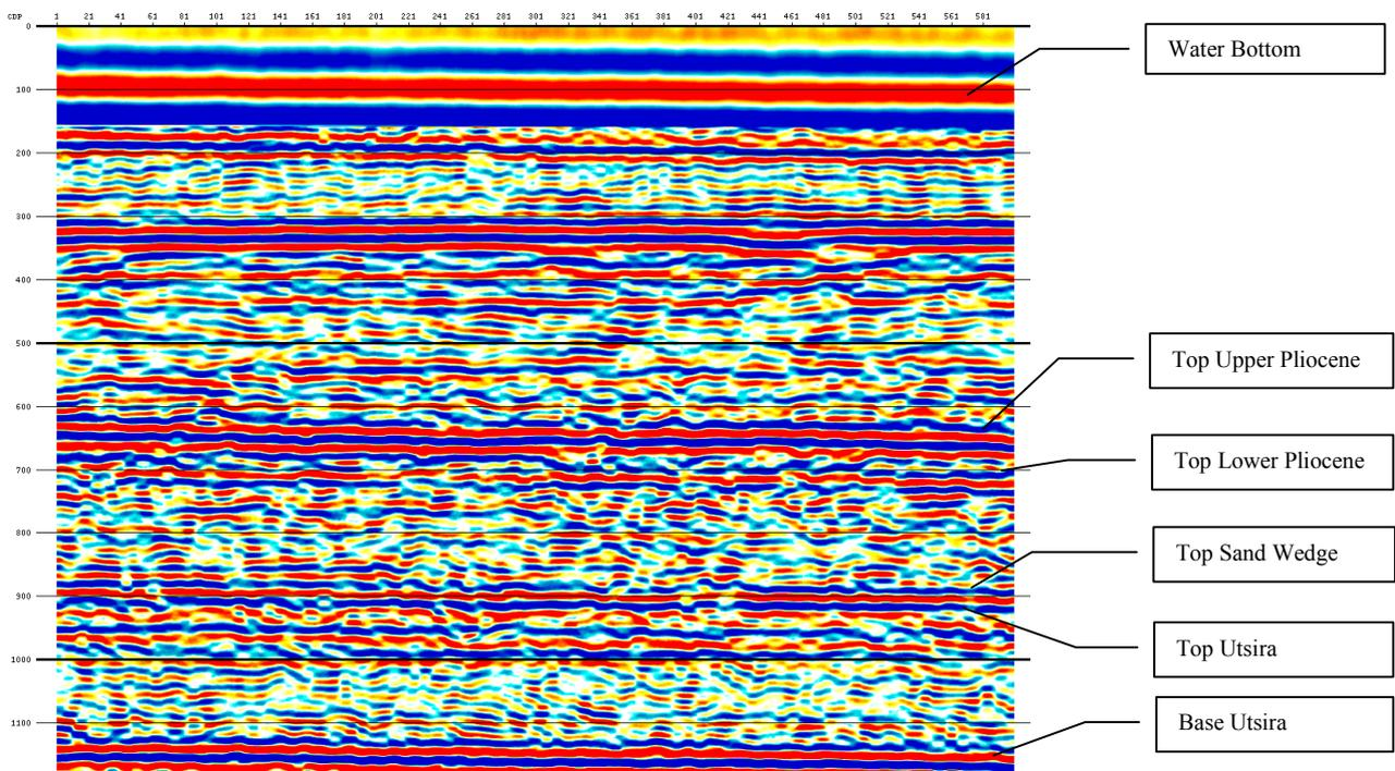
Figure 7.5 – 2-D seismic line (600 traces) recorded over the Sleipner overburden model. The horizons built within the model have been identified with the Base Utsira reflection recorded from the base of the steel water tank.
