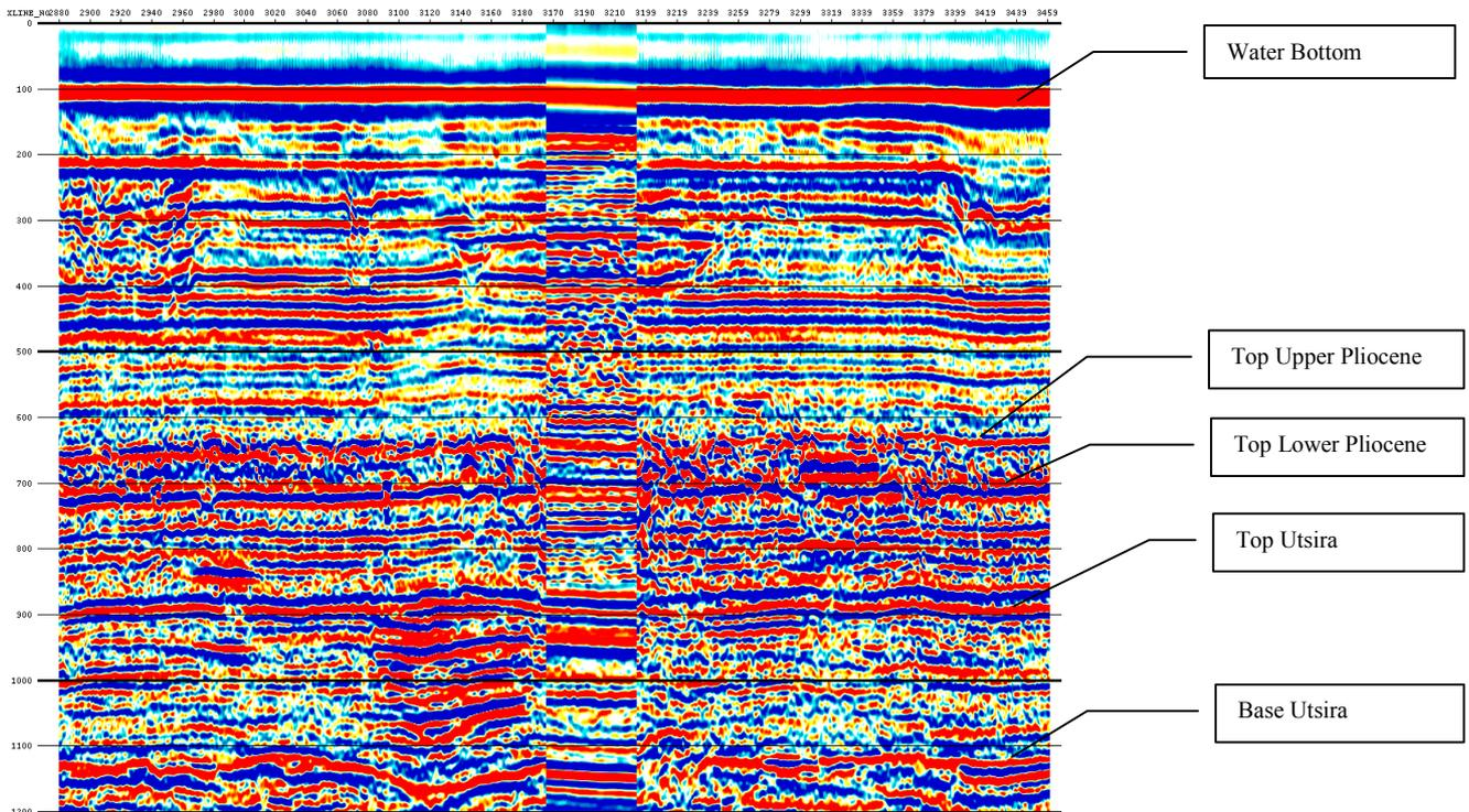
Figure 7.6 – Model stack inserted into field seismic Inline 3842 recorded in 1999 after approximately 3 million metric tonnes of CO<sub>2</sub> had been sequestered.
