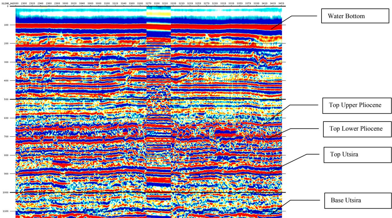
Figure 7.5 – Model stack inserted into field seismic Inline 3842 recorded in 1994. The CO<sub>2</sub> injection point is located to the left of the inserted model data.
