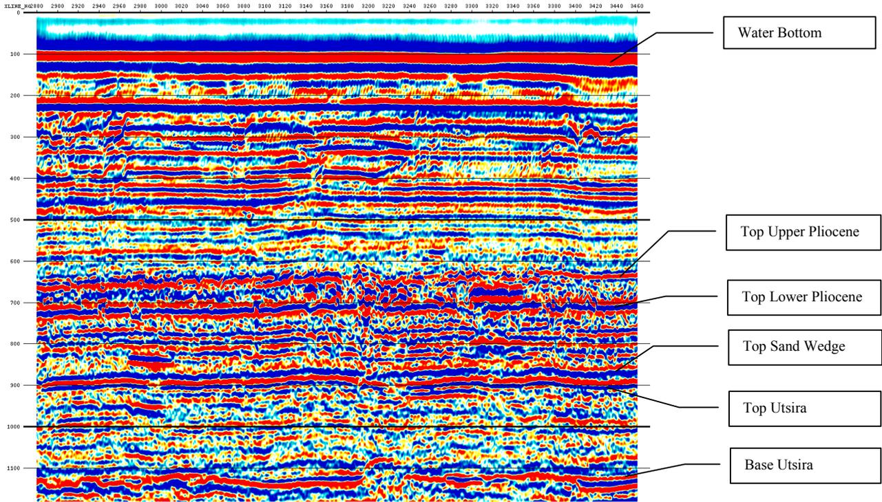
Figure 7.4 – Inline 3842 of the 1994 field seismic survey. The horizons incorporated into the Sleipner overburden model are the Top Pliocene, Top Lower Pliocene, Top Sand Wedge and Top Utsira horizons.
