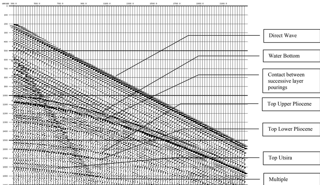
Figure 7.1 – An example of a typical raw model CMP gather with AGC applied. Reflection events were recorded from each interface within the model as well as other events such as the direct wave, multiples and an apparent coherent noise event associated with the source.
