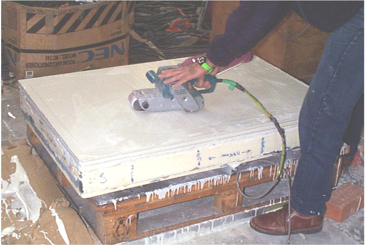
Figure 5.3 – After each layer in the Sleipner overburden model was formed, the layer was machined and sanded to give an even surface.
