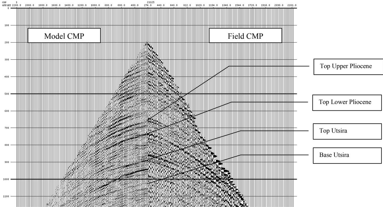
Figure 7.2 – The raw model CMP gathers were frequency filtered, true amplitude gain corrected, muted and then compared with the field CMP gathers from the 1994 survey. A typical model CMP gather is shown alongside a field CMP taken approximately 500 m NE of the CO<sub>2</sub> injection point.
