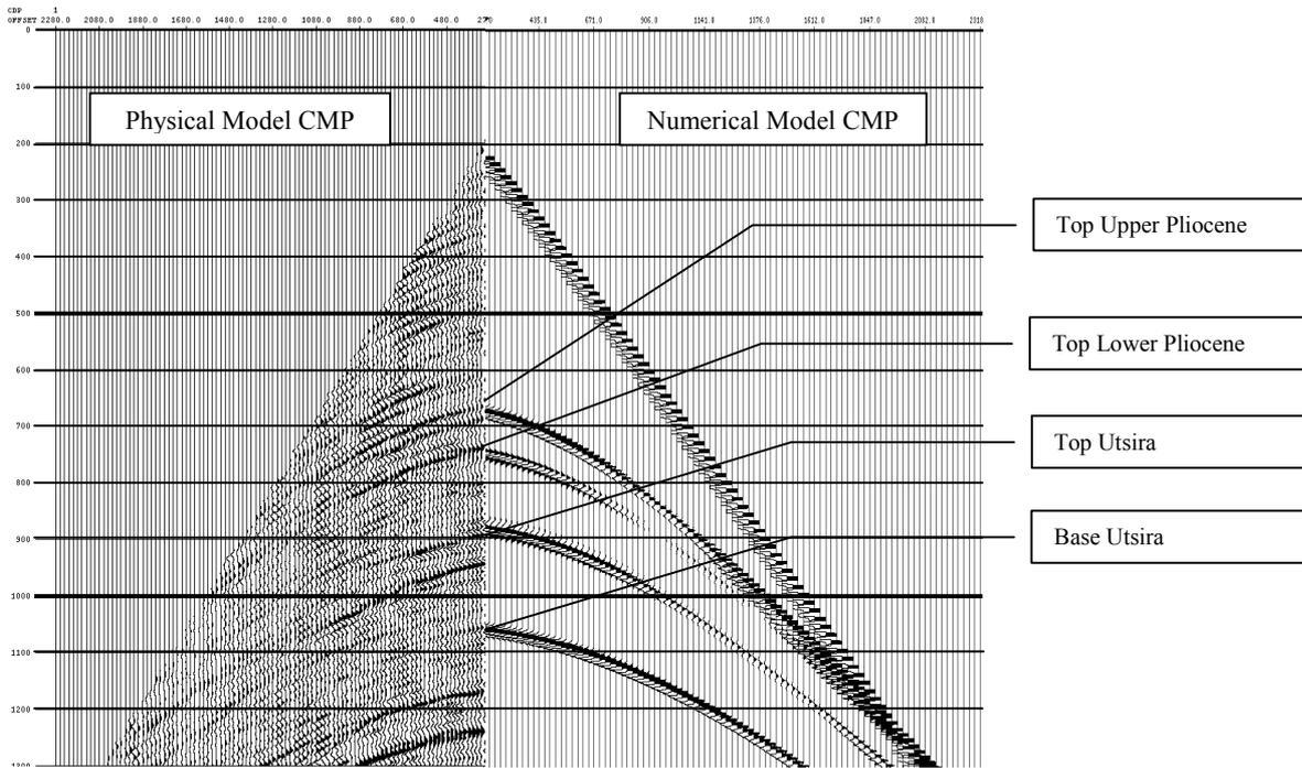
Figure 8.1 – A typical physical model CMP gather inserted alongside the numerical gather. The timing match of horizons and moveout between the physical model and the numerical data appears satisfactory.
