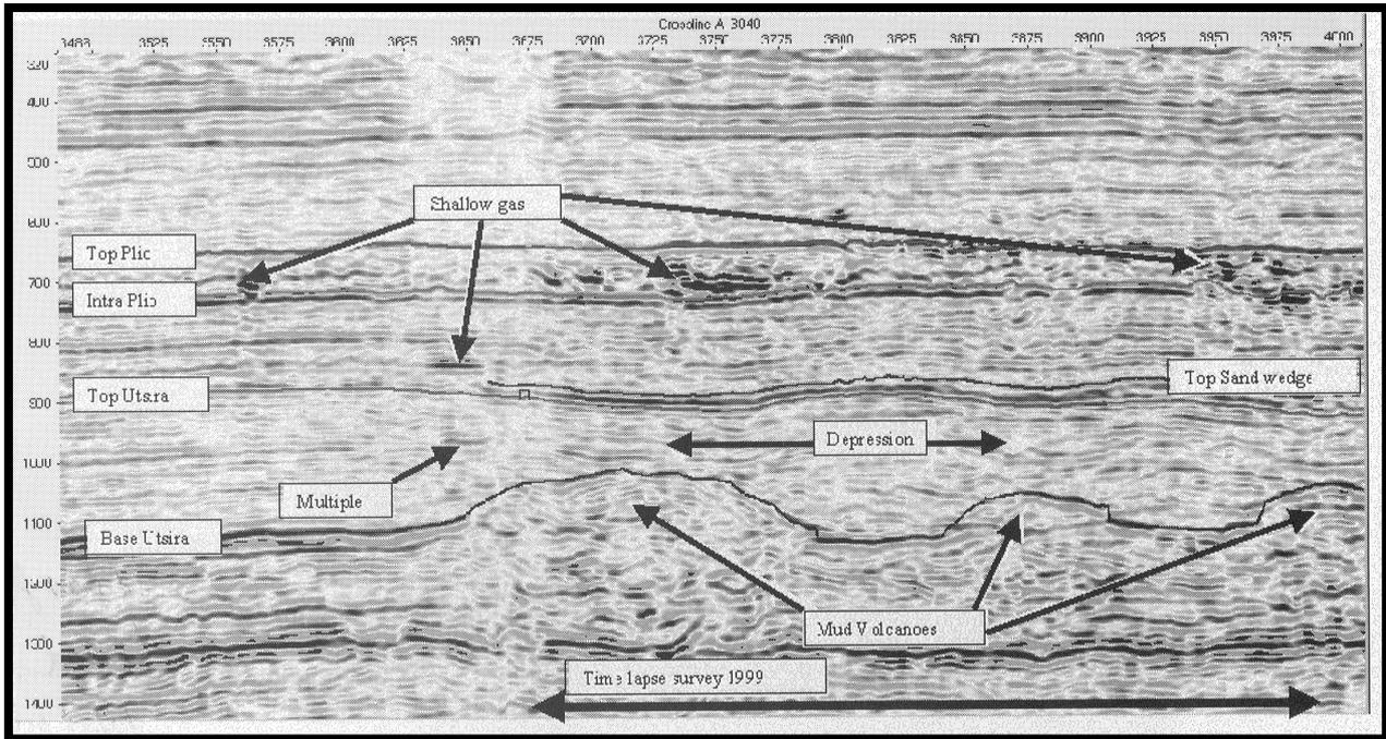
Figure 1 – The Nordland Shales and the Quaternary Sand units overlie The Utsira sand. The Nordland shales exhibit anomalously high reflection amplitudes that may be attributed to isolated high-velocity lithologies or the presence of shallow gas (after Arts et al., 2000).
