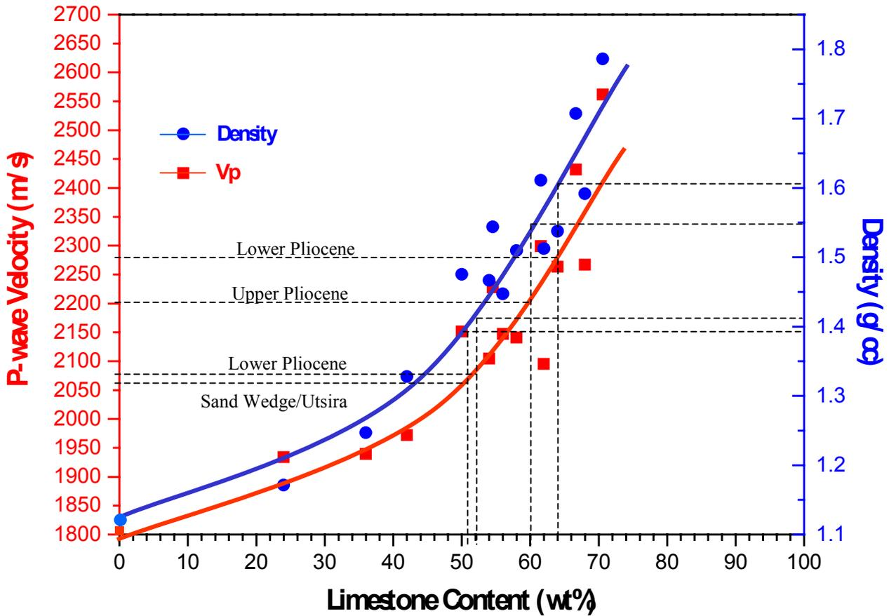
Figure 4.2 – Measured P-wave velocity and density values for each layer within the Sleipner overburden model. Parts A+B were mixed in equal amounts with limestone powder added to boost P-wave velocity and density (expressed as wt% of total mix). To match the Quaternary interval velocity, no limestone powder was added.
