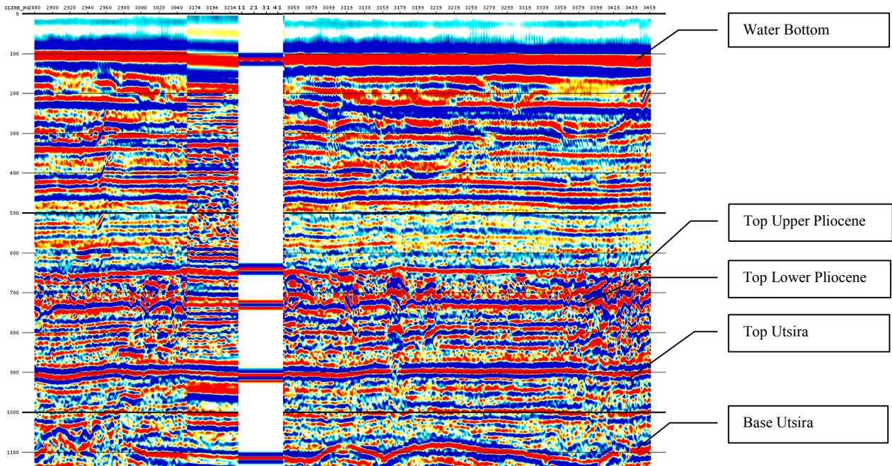
Figure 8.2 – Both physical and numerical model stacks inserted into field Inline 3780 recorded in 1994. The frequency content of the physical model and field data appear slightly lower than the numerical data, which is consistent with the higher frequency wavelet used in the numerical calculation.
