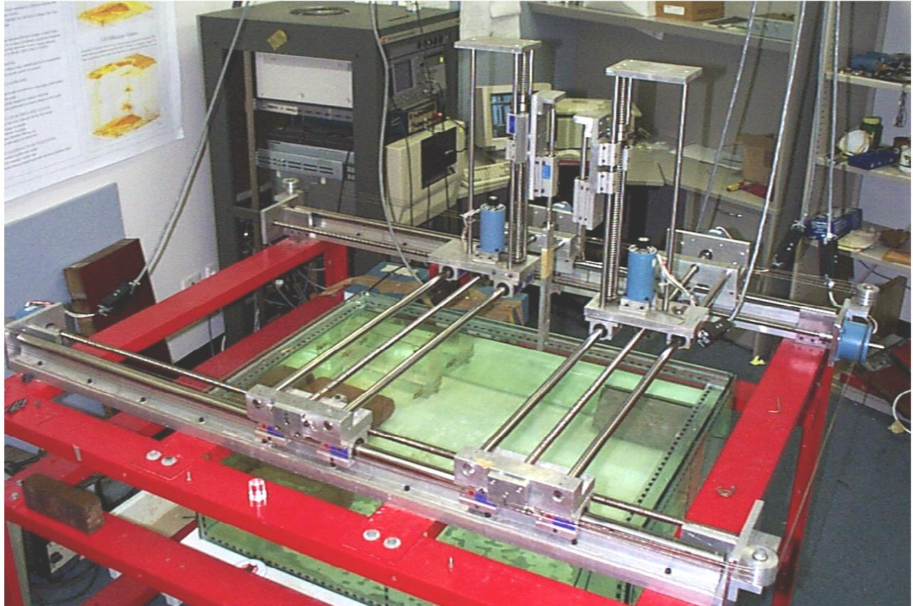
Figure 4.1 – Seismic physical modelling system at Curtin University of Technology, Perth, Australia. A PC controls the movement of simulated seismic sources and receivers within an  $x, y, z$  coordinate system. The signal output from the receiver is fed into a 12-bit A/D converter, which is stored to the hard disk of the PC and downloaded over the network to seismic workstations.
