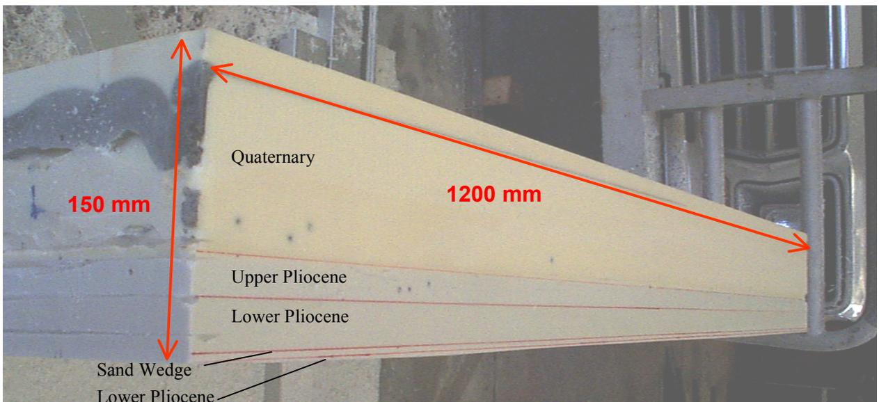
Figure 5.4 – The final Sleipner overburden model measured 1200 mm x 800 mm x 150 mm and weighed in excess of 250 kg. The model was placed in a steel tank filled with water to simulate marine seismic recording.
