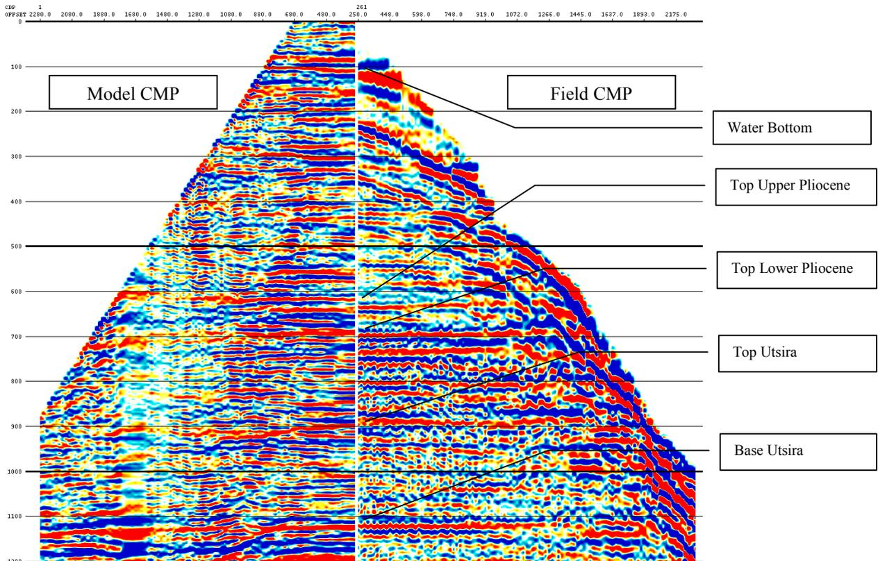
Figure 7.3 – Comparison between NMO corrected CMP gathers taken from both the model and 1994 field data.
