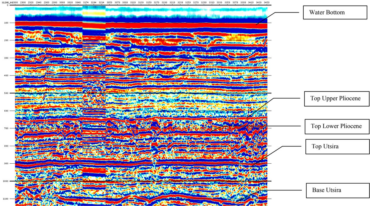
Figure 7.4 – A model stack consisting of 60 traces inserted into field Inline 3780 recorded in 1994. There are slight timing errors between some events and an almost perfect match between others. Overall, the frequency content between the two data sets appears very similar.
